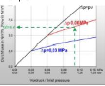
$QG = QD \times F$   $QG \blacktriangleright A = 6,4 \times 1,2 = 7,68 \text{ m}^3/\text{h} C_2H_2$  QG = flow / gas type F = conversion factorQD = flow / air
